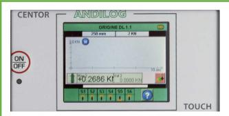
The Centor Star Touch screen is reversible without disassembly the gauge. it is possible to rotate by 90°, 180° or 270°.
