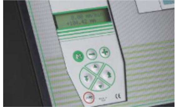
The manual motor command allows a smooth crosshead displacement to get into position before starting the measurements or to adjust first tests.
